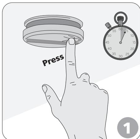
Press and hold the test button for a few seconds.
